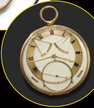
This pocket chronometer features Daniels's slim co-axial escapement and jumping seconds. At right is Daniels at his bench.
